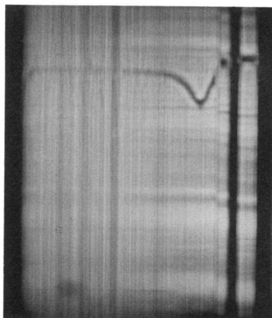
FIG. 4. Schlieren pattern of partition chromatography-purified protein-lipopolysaccharide complex. The photograph was taken 66 min after 20,410 rev/min was reached. The sample concentration was 5 mg/ml in 0.15 M NaCl.
