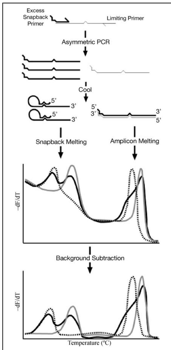
**Fig. 1. Snapback primer genotyping with a saturating DNA dye.**
