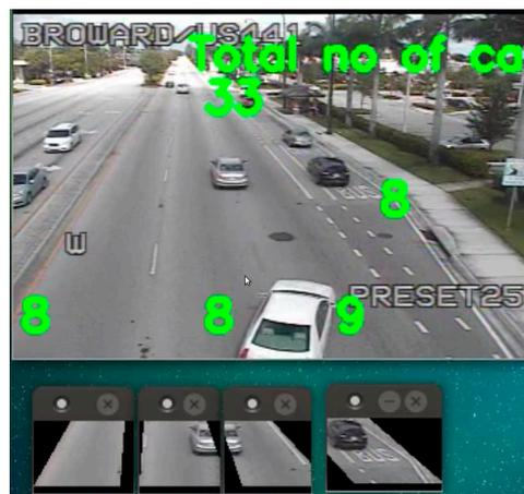
**Figure 9.** The double counting issue, when a car moves between two RIOs.
