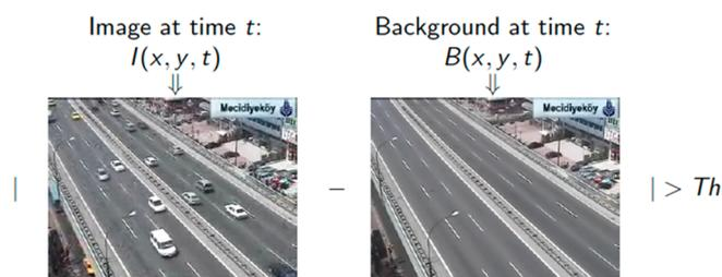
Figure 1. Basic approach of background subtraction method.
