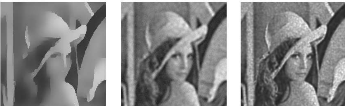
Figure 4: The restoration results by three models when m = 50 . Left: PM equation (3.2); Middle: YK equation (1.2); Right: our model (3.1).
