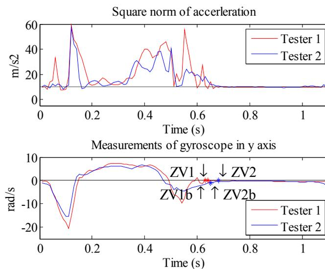
**Figure 10.** The square norm of acceleration and the gyroscope measurements in the  $y$  axis of two testers, and the comparison of ZV boundaries obtained by two methods
