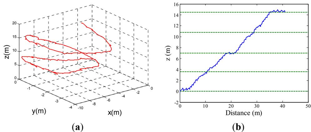
**Figure 17.** (a) Estimated 3D path for going upstairs; (b) Estimated altitude.
