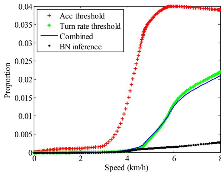
**Figure 12.** The proportion of ZV false detections in the total test duration with different methods at different speeds.
