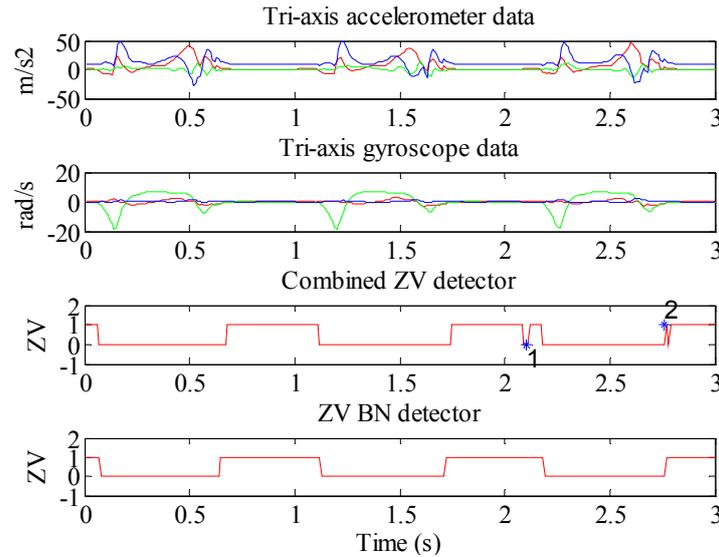
**Figure 11.** The comparison of ZV false detections between the combined condition method and the BN inference method.
