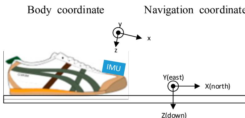
**Figure 2.** IMU installation mode and the relationship between body coordinate and navigation coordinate.
