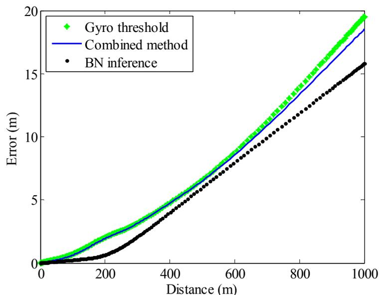
**Figure 14.** Average horizontal error by PINS/EKF based on different ZV detectors.
