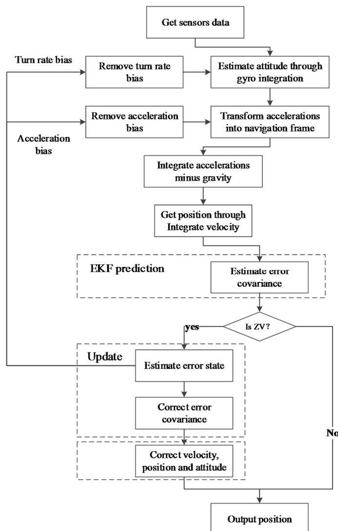
**Figure 8.** The EKF framework used for PINS.
