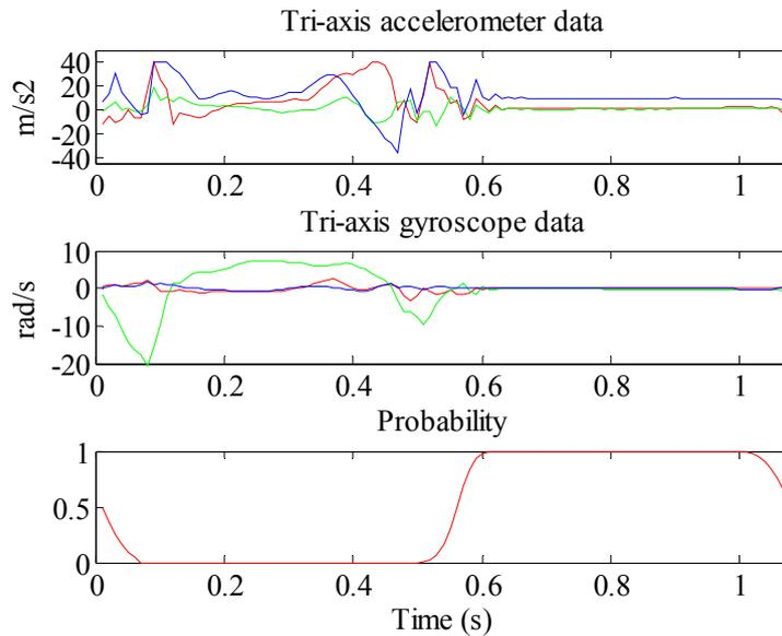
**Figure 7.** Measurements of accelerometer and gyroscope in one gait cycle, and CPD in measurement cycle.
