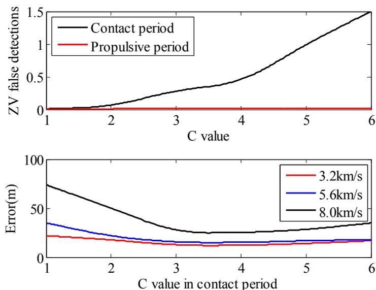
**Figure 9.** The average ZV detections in the contact period and propulsive period with different C values in Formula (11) and horizontal position errors with different C values in the contact period.
