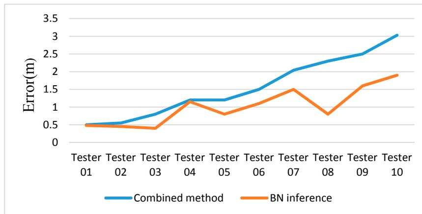
**Figure 13.** Experiment results of altitude error in a total distance of 100 m with ten testers at normal speed.
