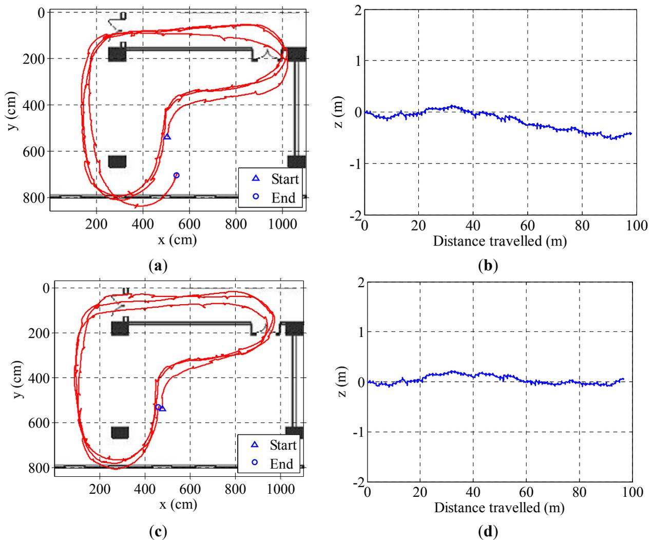
**Figure 15.** The comparison of the tracking results based on different ZV detectors. (a) Estimated 2D path based on the combined condition method; (b) Estimated altitude based on the combined condition method; (c) Estimated 2D path based on the BN method; (d) Estimated altitude based on the BN method.
