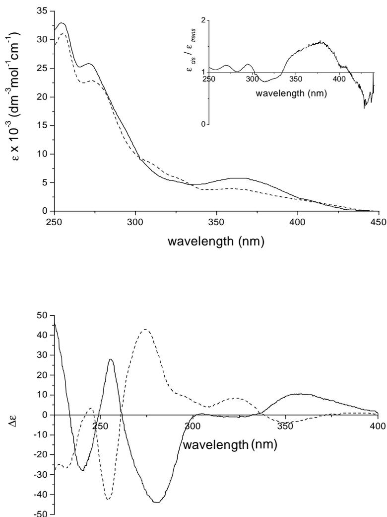
**Figure 2.1** UV-VIS (top) and CD (bottom) absorption spectra of donor-acceptor switch **2.2** together with the ratio of the two extinction coefficients ( $\epsilon_{\text{cis}} / \epsilon_{\text{trans}}$ , inset). The solid lines correspond to (*M*)-*cis*-**2.2** and the dashed graphs to (*P*)-*trans*-**2.2**.
