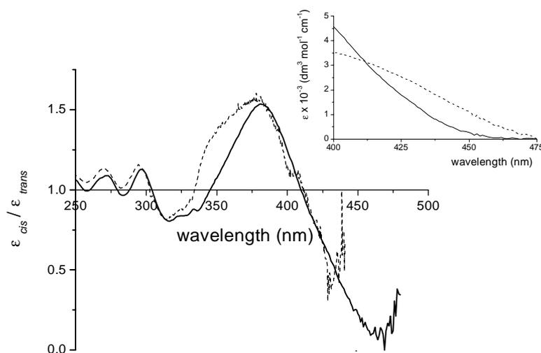
**Figure 2.7** Ratio of extinction coefficients for the *cis*- and *trans*-form of compound **2.4** (solid curve, the ratio found for compound **2.2** is given as a comparison (dashed curve)). The inset shows the red-end of the absorption spectrum for the *cis*- (solid) and *trans*- (dashed) form of **2.4**.
