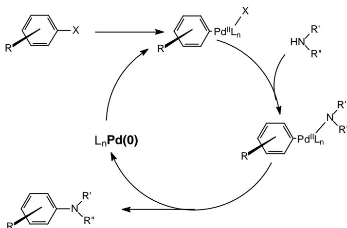
**Scheme 2.8** Catalytic cycle for Pd-catalyzed amination of arylhalides (adapted from ref. 21).
