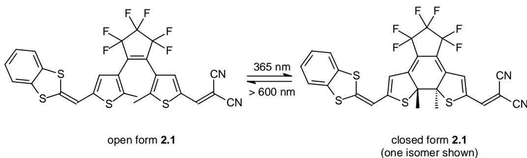
**Scheme 2.1** A donor-acceptor substituted diarylethylene switch.
