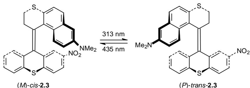
**Scheme 2.3** Alternative chiroptical molecular switch **2.3** with donor in upper half and acceptor in lower half of the molecule.
