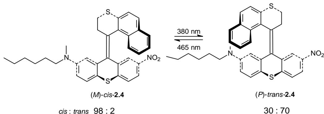
**Scheme 2.13** Highly efficient chiroptical molecular switch **2.4**.
