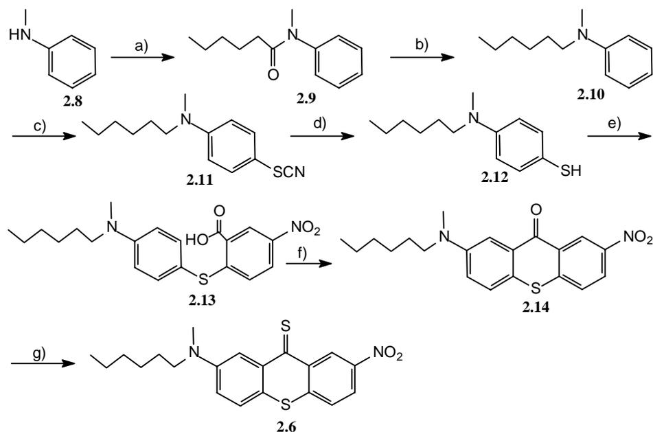
**Scheme 2.7** Formation of thioketone **2.6** in a linear approach towards compound **2.4**: a) hexanoyl chloride, 86%, b)  $\text{BH}_3$  / THF,  $\Delta$ , 77%, c) KSCN, AcOH,  $\text{Br}_2$ , 86%, d)  $\text{Na}_2\text{S}$ , NaOH, EtOH,  $\Delta$ , yield not determined, e) 2-chloro-5-nitro benzoic acid, KOH, EtOH,  $\Delta$ , 94% (over two steps), f) polyphosphoric acid,  $130^\circ\text{C}$ , 56%, g) Lawesson's reagent, toluene,  $\Delta$ , 73%.
