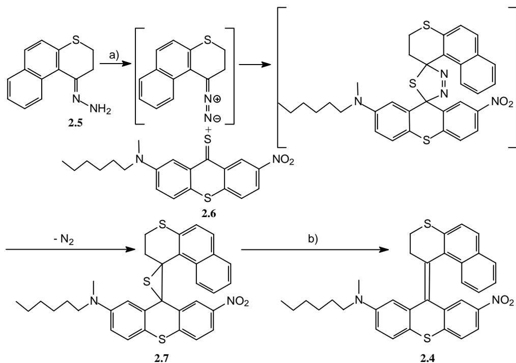
**Scheme 2.6** The diazo-thioether coupling illustrated for compound **2.4**: a)  $Ag_2O$ ,  $MgSO_4$ ,  $KOH/MeOH$ ,  $CH_2Cl_2$ ,  $-10 - 0^\circ C$ , 85%, b)  $Cu$ , *p*-xylene,  $\Delta$ , 79%.
