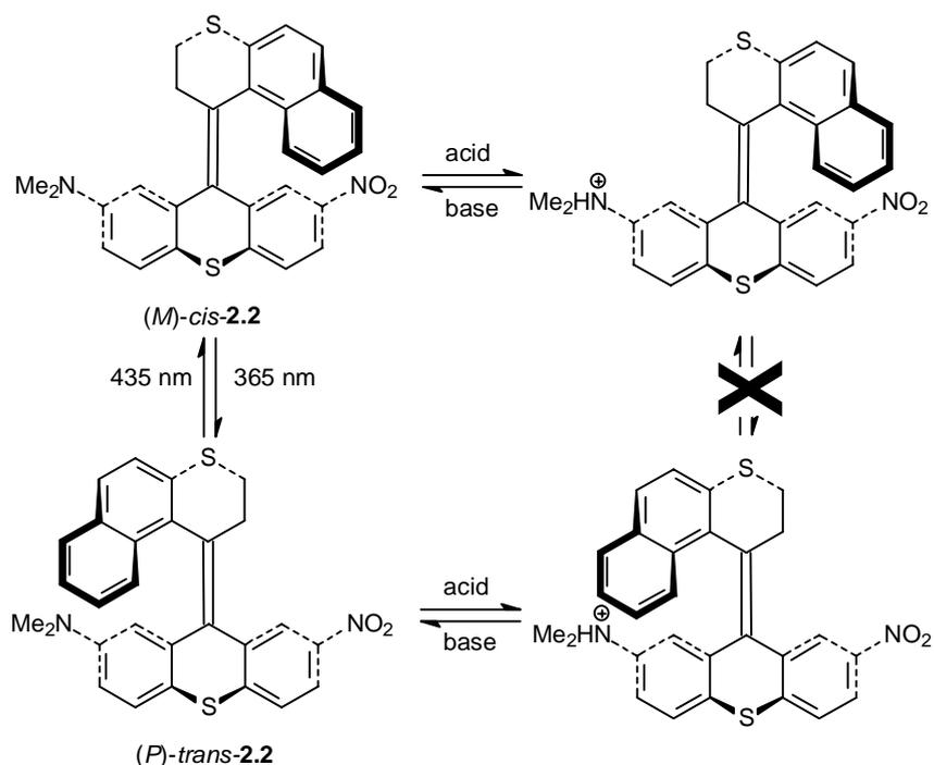
**Scheme 2.4** Blocking isomerization by protonation allowing gated photoswitching.
