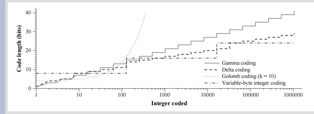
Code lengths in bits of Elias gamma and delta codes, a Golomb code with k = 10, and variable-byte integer codes for integers in the range 1 to around 1 million
