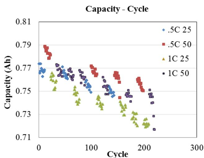
The objective of our experiment was to simulate the application under the combined factors. The conditional parameters are listed in Table 2. As Figure 4 shows, the capacity profile moved up with a higher temperature under the same discharge rate, while it went down with a higher discharge rate at the
