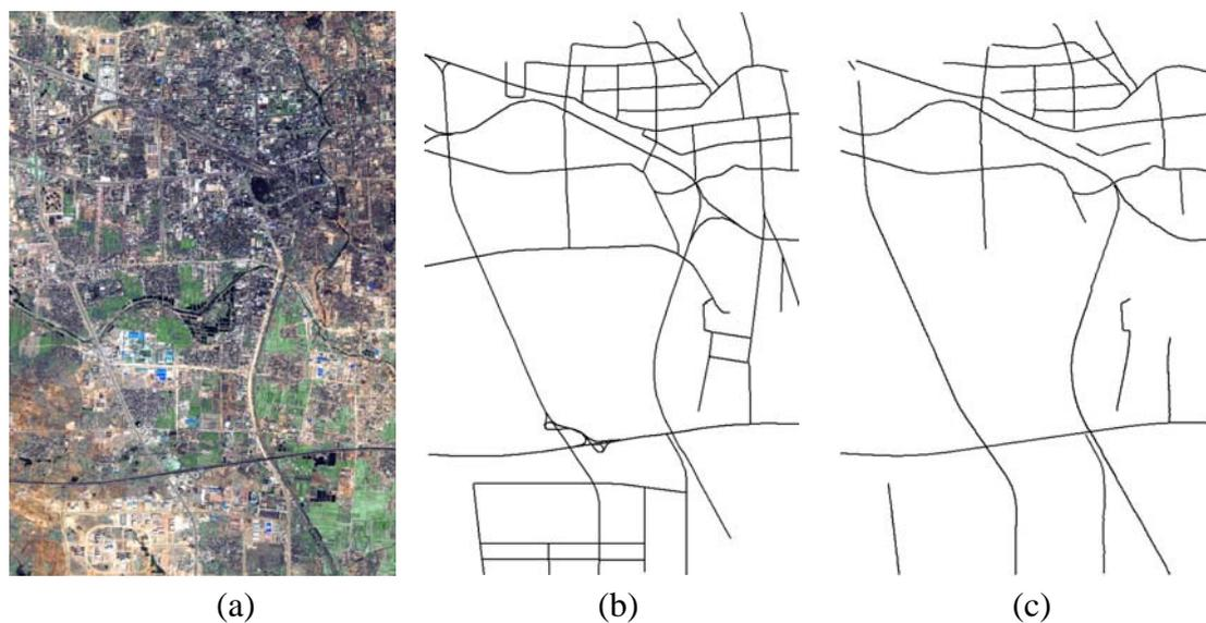
**Figure 5.** Road network extraction from a QuickBird satellite image. (a) QuickBird fused image with  $0.61 \text{ m pixel}^{-1}$  resolution and the image size is 15,368 pixels by 10,240 pixels; (b) the reference road network plotted; (c) the extracted vector road network by the combination strategy.
