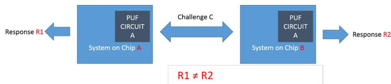
**Figure 1.** Two identical physical unclonable functions (PUFs) circuits on two different chips generate different responses.
