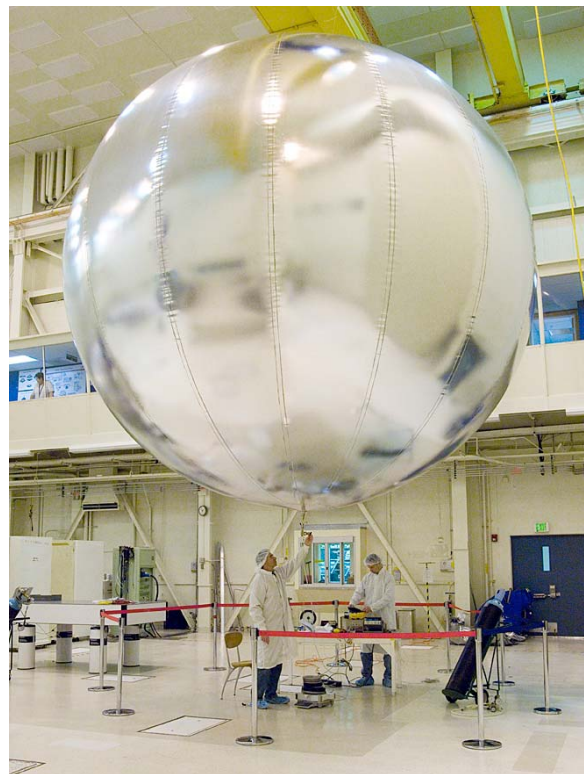
Fig 1. Prototype Venus Balloon During Testing
