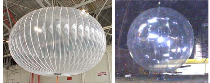
Fig 4. Pumpkin and Spherical Superpressure Balloons
