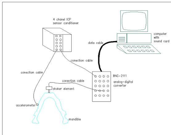
Figure 1: Experimental device for damping measurement.
