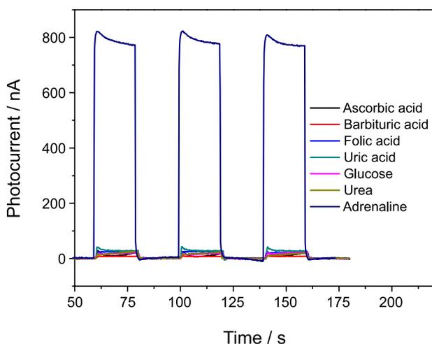
**Figure 7.** Photocurrent obtained for proposed photoelectrochemical sensor toward several foreign species in comparison to that obtained for adrenaline under optimized conditions at an applied potential of 0.4 V vs. Ag/AgCl. The concentration of all species was fixed at 100  $\mu\text{mol L}^{-1}$ .
