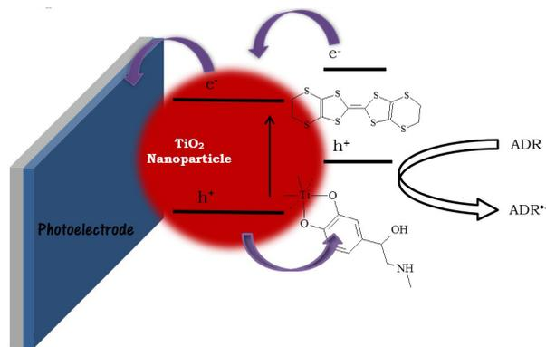
**Figure 2.** Proposed mechanism for the photoelectrochemical detection of adrenaline.
