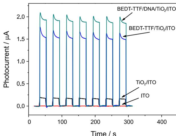
**Figure 1.** Photocurrent response of BEDT-TTF/DNA/TiO<sub>2</sub>/ITO, BEDT-TTF/TiO<sub>2</sub>/ITO, TiO<sub>2</sub>/ITO, and ITO. Experiments carried in 0.1 phosphate buffer solution (pH 7.0) containing 1 mmol L<sup>-1</sup> adrenaline.  $E_{app} = 0.25$  V vs. Ag/AgCl.
