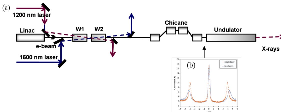
The effect of a linear energy chirp on FEL amplification has been studied and a new proposal of using a tapered undulator was made, showing the generation of 200 attoseconds X-ray pulses with a power of 100 GW [37].
