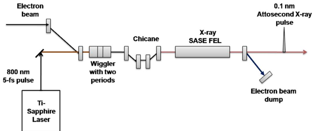
In our study, the laser wavelengths, FWHM pulse duration and electron bunch energy distributions were optimized to control the side current peaks and to obtain a single isolated attosecond pulse.
