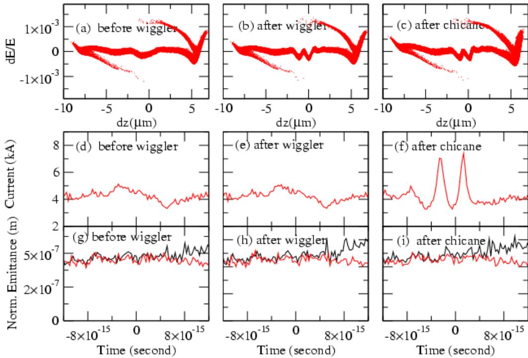
**Figure 10.** (Color online). The change of the characteristics of the 6 kA, 12  $\mu\text{m}$ -long electron bunch. (a)–(c): the longitudinal energy distribution. (d)–(f): current profile. (g)–(i): horizontal (black line) and transverse normalized-emittance (red line)[42].
