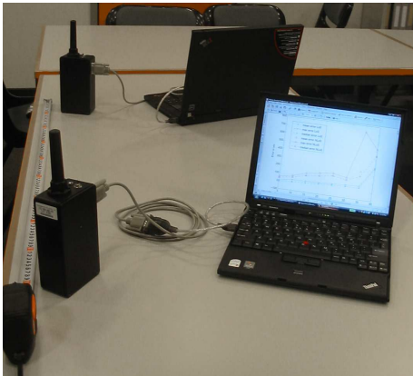
Fig. 4. The implementation setup for the authenticated ranging system.
