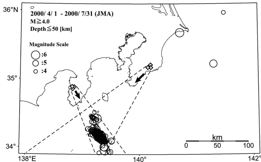
**Figure 8.** Triangulation of the noise source (#4 in Fig. 6) by using the azimuths estimated from the Izu and Boso peninsula arrays.
