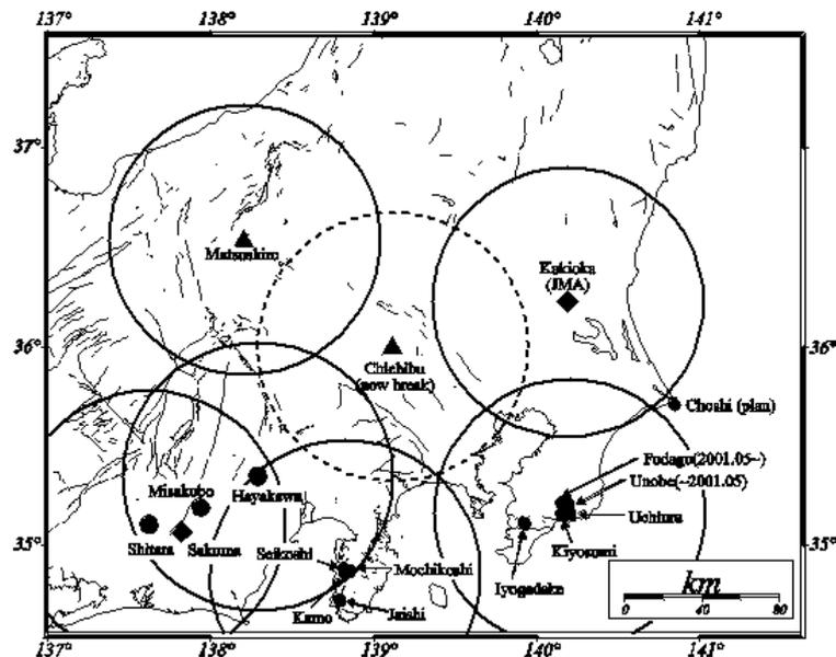
**Figure 3.** A ULF network in the Kanto (Tokyo) area. A triangle indicates the installation of an induction magnetometer and a circle, the torsion-type magnetometer. Kakioka observatory is equipped with induction magnetometers. A box indicates the fluxgate magnetometer.
