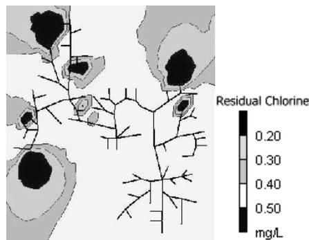
Fig. 4 – Concentration tie-lines of chlorine throughout the system (12 hours)
