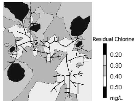
Fig. 5 – Concentration tie-lines of chlorine throughout the system (12 hours)
