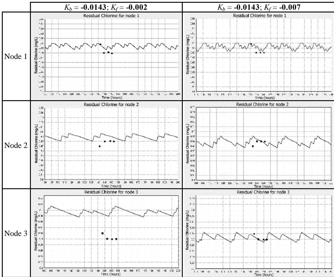
Fig. 6 – Simulation results for nodes 1, 2 and 3, before and after  $K_f$  calibration
