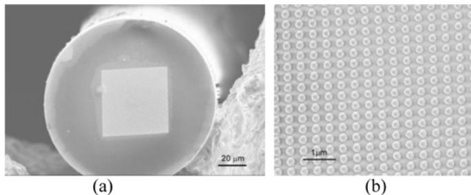
Fig. 1. Scanning electron micrographs of a gold nanodot array on an optical fiber tip. (a) Overview of the optical fiber end facet, and (b) the gold nanodot array on the optical fiber facet.
