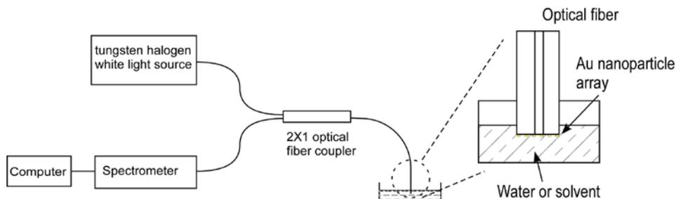
Fig. 2. Optical setup for the fiber tip LSPR sensor based on reflection spectra measurement.
