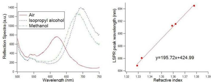
Fig. 4. (a) Measured transmission spectra for the fiber sensor in various solvents. (b) Dependence of the LSPR peak wavelength on the index of refraction of the solvents, methanol (1.329), water (1.333), acetone (1.359), ethanol (1.362), and isopropyl alcohol (1.378).
