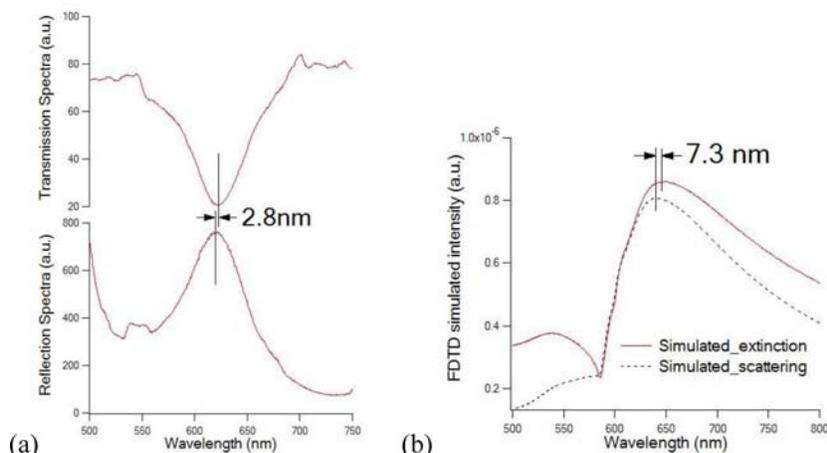
Fig. 3. (a) The transmission spectrum (top) and reflection spectrum of the fiber tip LSPR sensor in the air, and (b) the calculated spectra for extinction (solid line) and scattering (dash line) for the LSPR on the gold nanodot array.
