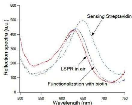
Fig. 5. The reflection spectra of the Au nanodots array on the optical fiber end facet when it is in air (red solid curve), functionalized with biotin (blue dotted curve), and bound with streptavidin (green dash-dot curve). Plasmonic peaks shift due to the functionalization of biotin and specific binding of streptavidin can be clearly observed.
