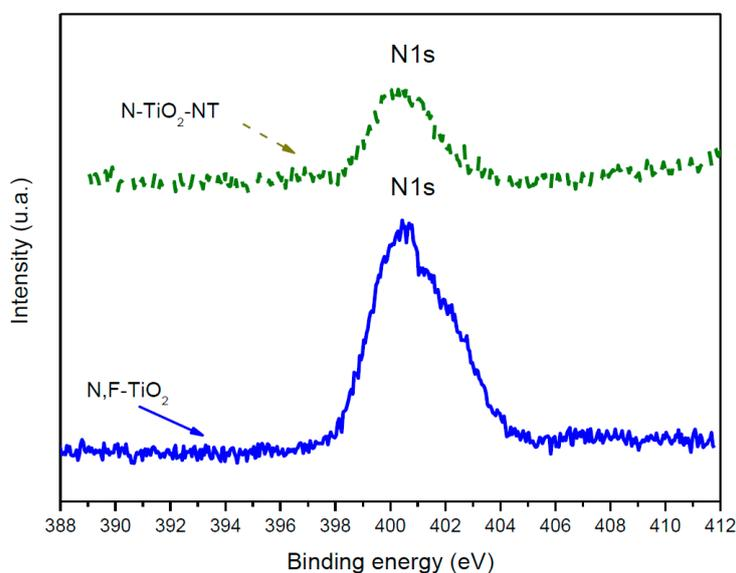
**Figure 2.** XPS spectra of the N 1s core level obtained for N,F-TiO<sub>2</sub> and N-TiO<sub>2</sub>-NT.
