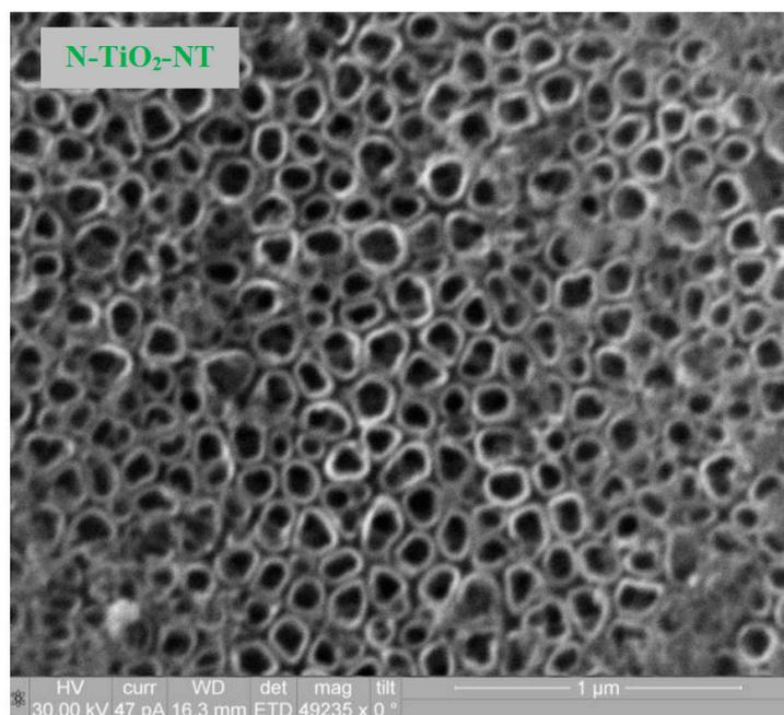
**Figure 1.** SEM image of titania nanotubes (N-TiO<sub>2</sub>-NT) grown by anodization of Ti foil, followed by annealing in ammonia atmosphere.
