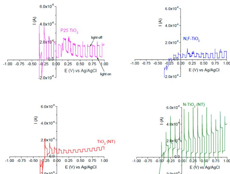
**Figure 5.** Linear sweep voltammograms for nanoparticle (P25 and N,F-TiO<sub>2</sub>) and nanotube (TiO<sub>2</sub>-NT and N-TiO<sub>2</sub>-NT) electrodes in  $\frac{1}{4}$  strength solution under chopped visible irradiation (10 s light on/off). The potential was swept positive at a sweep rate of 5 mV s<sup>-1</sup>.
