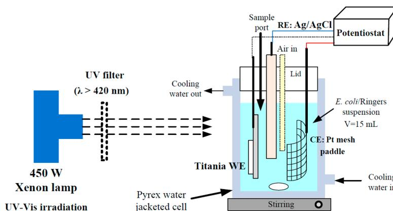
Figure 8. Photoelectrochemical cell.
