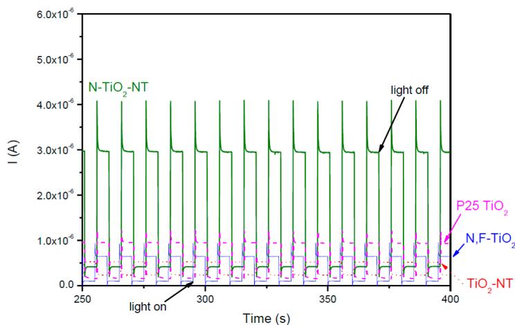
**Figure 6.** Current-time behavior of nanotube (TiO<sub>2</sub>-NT and N-TiO<sub>2</sub>-NT) and nanoparticle (P25 and N,F-TiO<sub>2</sub>) electrodes in  $\frac{1}{4}$  strength solution under chopped visible irradiation (light on/off 10 s) at fixed potential (+1.0 V). Data shown is from the third cycle of current measurement for each electrode.
