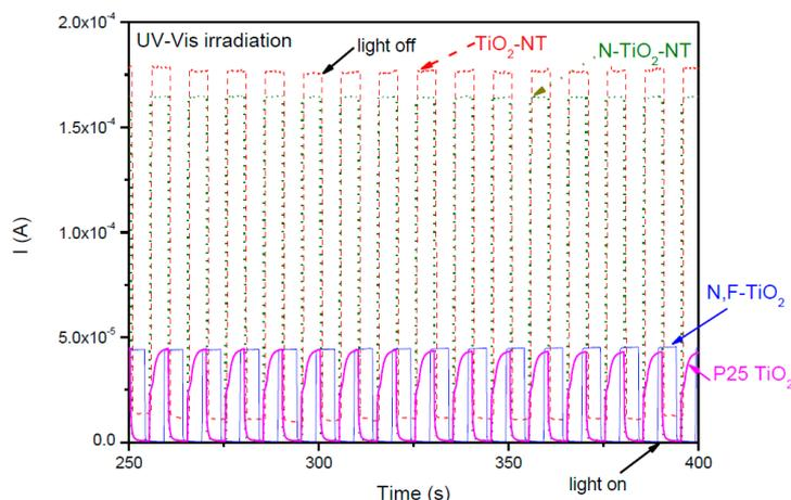
**Figure 4.** Current-time behavior of nanotube (TiO<sub>2</sub>-NT and N-TiO<sub>2</sub>-NT) and nanoparticle (P25 and N,F-TiO<sub>2</sub>) electrodes in  $\frac{1}{4}$  strength solution under chopped UV-Vis irradiation. UV-Vis exposure time: 5 s. Potential bias: +1.0 V. 3rd cycle of current measurement for each electrode.
