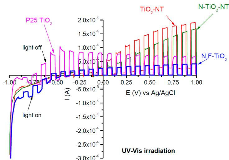
**Figure 3.** Linear sweep voltammograms for nanotube ( $\text{TiO}_2\text{-NT}$  and  $\text{N-TiO}_2\text{-NT}$ ) and nanoparticle (P25 and  $\text{N,F-TiO}_2$ ) titania electrodes in  $\frac{1}{4}$  strength solution under chopped (10 s light on/ off) UV-Vis irradiation. The potential was swept from negative to positive with a sweep rate of  $5 \text{ mV s}^{-1}$ .
