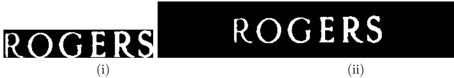
Figure 8. Postprocessing the binarized image by padding background pixels to eliminate foreground-background ambiguity. (i) The text connected components touch the boundary. (ii) Foreground and background are clearly separated, after background padding.
