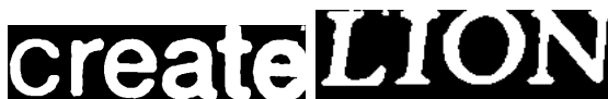
Figure 6. Word images shown in Fig 5, after segmentation by our algorithm using the plane with maximum discrimination factor, computed post non-linear enhancement.
