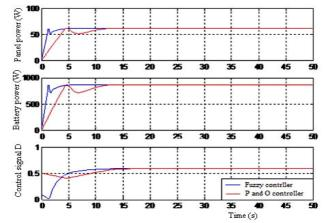
Fig. 9: Variation of the panel power, battery power and the duty ratio D, under standard conditions: temperature (25 °C) and solar insolation (1000 W/m<sup>2</sup>)
