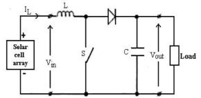
Fig. 6: Basic circuit of the boost chopper
