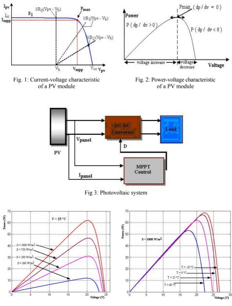
Fig. 4: Influence of the solar radiation for constant temperature
