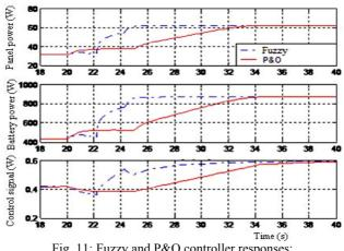
Fig. 11: Fuzzy and P&O controller responses: for a fast solar insolation increase (500 W/m<sup>2</sup> to 1000 W/m<sup>2</sup> in 5 s at 25 °C)
