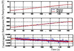
Fig. 15: Fuzzy and P&O controller responses: for a slow (120 s) temperature increase (20 °C to 30 °C) at 1000 W/m<sup>2</sup> of solar insolation
