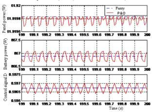
Fig. 10: Wave shape in steady state of the panel and battery power and of the duty ratio signals for a sampling rate of 100 Hz (T = 25 °C and S = 1000W/m<sup>2</sup>)
