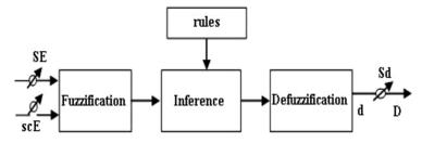
Fig. 7: General diagram of a fuzzy controller
