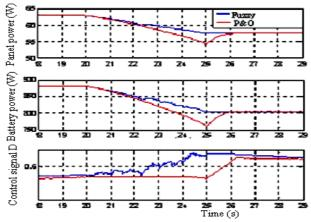
Fig. 17: Fuzzy and P&O controller responses: for a fast (5 s) temperature increase (20 °C to 45 °C) at 1000 W/m<sup>2</sup> of solar insolation
