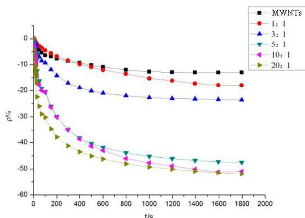
The different sensor response results of mixed ratios are shown in Figure 7. At a mass ratio of 10:1, the resistance-change rate of the adsorbent-mixed MWNT sensor to SO<sub>2</sub> is significantly greater than that of other ratios. At mass ratios of 5:1, 10:1, and 20:1, the resistance-change values of the adsorbent-mixed MWNT sensors to H<sub>2</sub>S were all large. Thus, sensors with different mixed ratios were selected to determine the selectivity of the two gases according to this feature.
