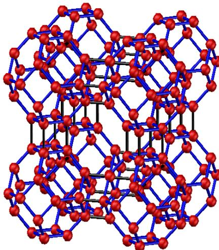
In the tetrahedral framework structure of zeolite, aluminum is trivalent, and four oxygen atoms surround an aluminum atom. That is, the aluminum-oxygen tetrahedron has a negative charge. To maintain the charge balance, metal cations offset the negative charge. The metal cations in 4 Å zeolite are sodium ions. The sodium ions and oxygen atoms form a stable structure.
