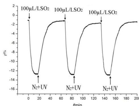
As shown in Figure 12, the desorption process enables the sensor resistance value to return to the initial value after testing. Many times during the tests, the resistance-change trends remained the same, whereas the maximum change rate remained similar and stable. In sum, the gas sensor may be used repeatedly to detect gases with good stability and reproducibility.
