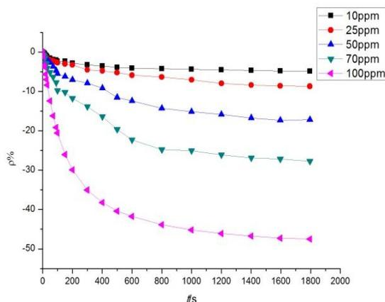
**Figure 11.** Linear relationship of MWNT sensor gas sensing response with different concentrations of SO<sub>2</sub> and H<sub>2</sub>S.
