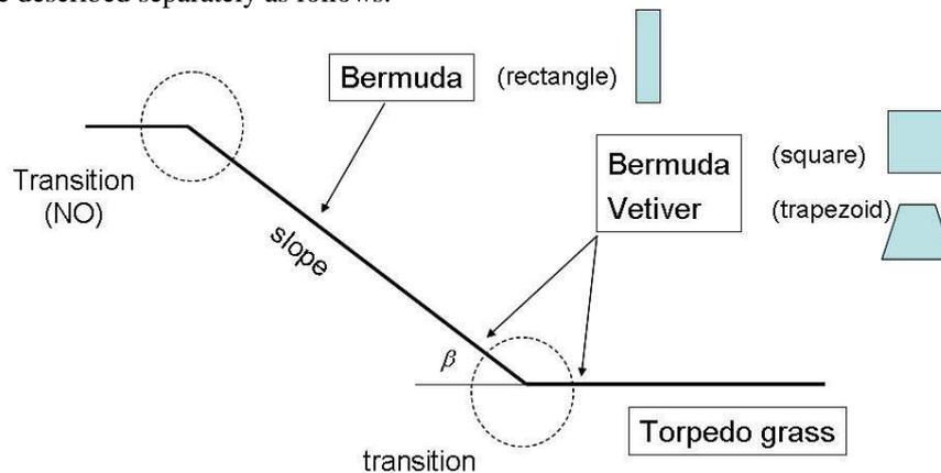
Figure 5. Damage positions and corresponding shapes.
