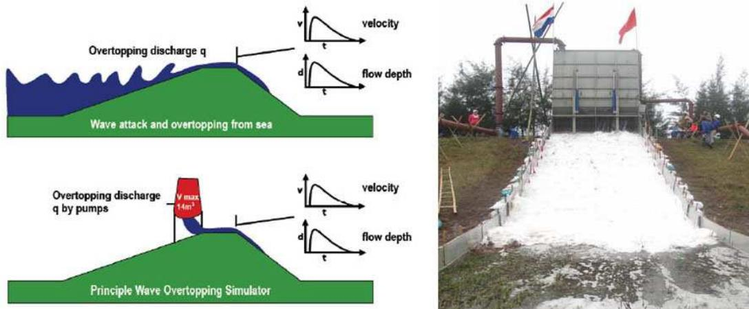
Figure 1. Left: principle of the Wave Overtopping Simulator. Right: overtopping flow released from the Simulator.
