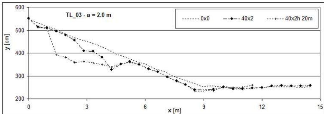
Figure 16. Grass slope profiles under attack of wave overtopping flow, centre cross-section with distance to both side walls of 2 m. Test location TL\_03 in Nam Dinh.
