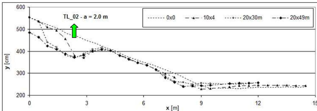
Figure 15. Grass slope profiles under attack of wave overtopping flow, centre cross-section with distance to both side walls of 2 m. Test location TL\_02 in Nam Dinh.
