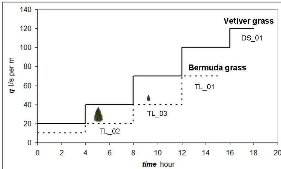
Figure 19. Maximum overtopping discharges on grass slopes.
