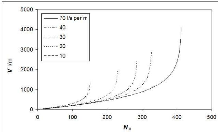
Figure 4. Distributions of overtopping wave volumes with different values of mean overtopping discharge.
