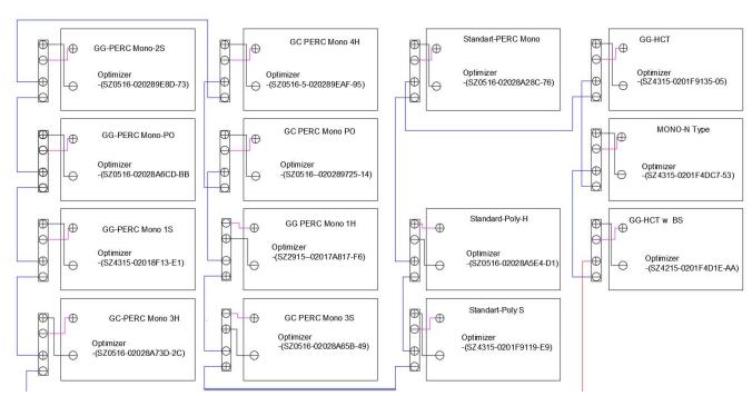
Fig. 1 The diagram of site setup and connections for modules under study.
