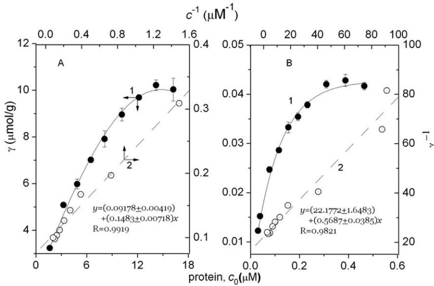
**Figure 2. Variation of  $\gamma$  of proteins in the presence of nano-HA.** 1:  $\gamma$  of cyt c (a) and hb (b) in the presence of nano-HA. a- the suspensions containing 500 mg/L nano-HA and 10 to 200 mg/L cyt c and b- 2500 mg/L nano-HA and 20 to 300 mg/L hb. All of the liquids were at pH 7.4 in 0.15 M NaCl. 2: Plots  $\gamma^{-1}$  vs.  $c_0^{-1}$  of the above liquids. doi:10.1371/journal.pone.0032818.g002
