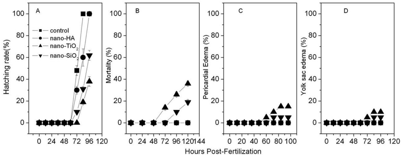
**Figure 7. Toxicity-causing rate of Zebrafish embryos and larvae.** A: Hatching rate, B: Mortality, C: PE and D: YSE. Exposed in 100 mg/L nano-HA, 100 mg/L nano-TiO<sub>2</sub> and 100 mg/L nano-SiO<sub>2</sub>. doi:10.1371/journal.pone.0032818.g007
