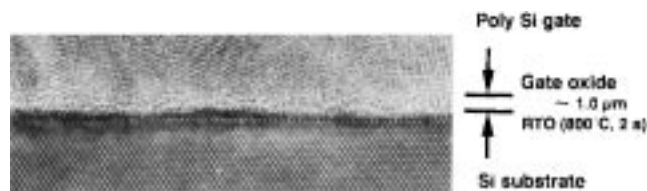
Fig. 7. TEM cross section of oxide film early in the oxidation process (2 s after the start of RTO at 800 °C).
