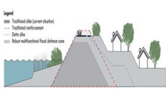
Figure 1. Dimension variation in representative cross section for the different multifunctional flood defence proposed solutions. (extracted from van Loon-Steensma and Vellinga (2014)).
