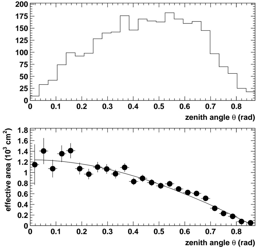
Figure 4: (a) Histogram of detected  $\gamma$ -rays as a function of incident zenith angle  $\theta$  for 10 GeV  $\gamma$ -rays. (b) Effective  $\gamma$ -ray detection area  $A(E, \theta)$  versus zenith angle at 10 GeV.
