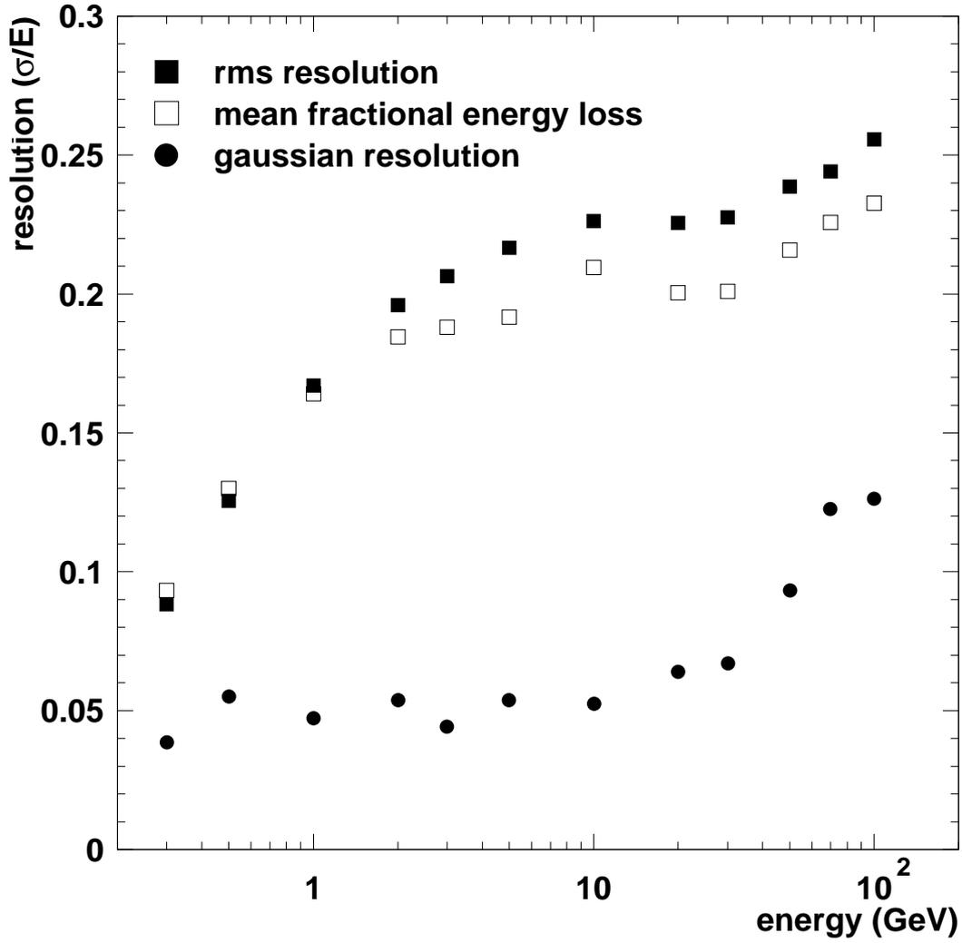
Figure 9: The mean fractional energy loss (open square), rms energy resolution (filled square), and width of the “gaussian” peak of the distribution (filled circle) as a function of primary  $\gamma$ -ray energy.
