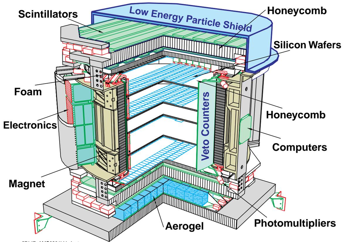
Figure 1: A cross section of the AMS instrument.
