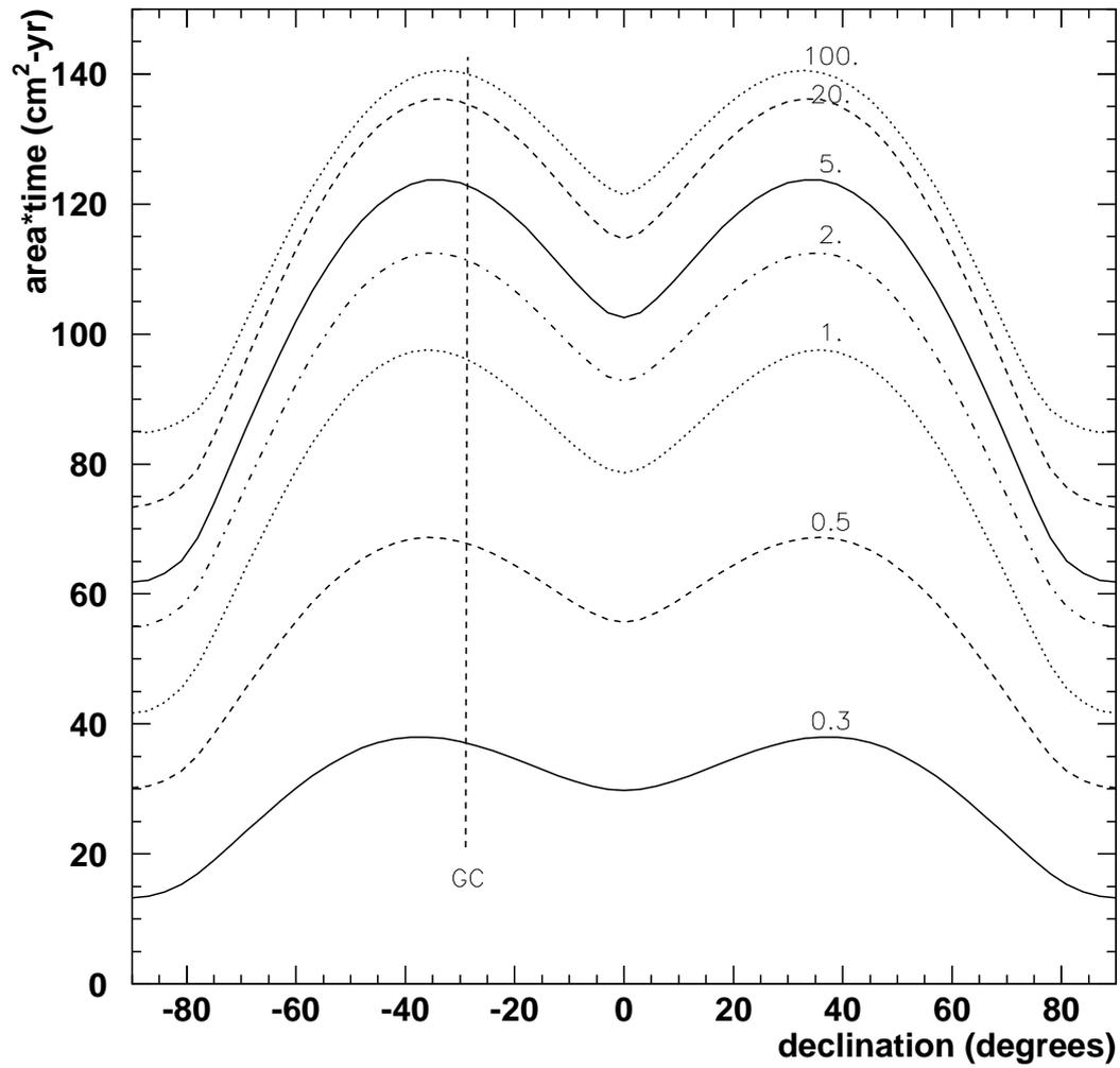
Figure 6: Accumulated area\*time product over one year of AMS operation as a function of declination; each curve is marked by the  $\gamma$ -ray energy (in GeV). The declination of the Galactic Center (GC) is also indicated as a dashed vertical line.
