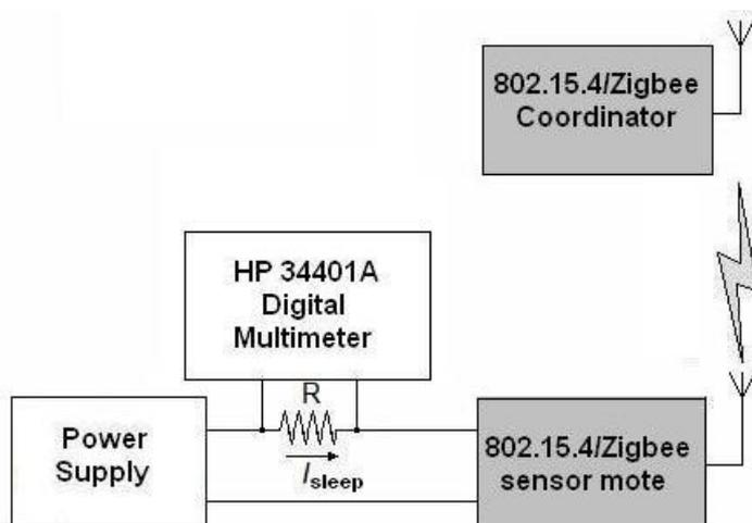
With this new testbed, the measured constant voltage in the resistor was estimated to be 24  $\mu$ V, which indicates that current absorbed by the mote is about 750 nA. The measurements for all the described operations of the mote have been tabulated in the Table 1.
