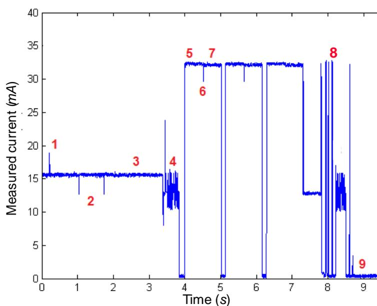
Interval 4: After the role of the mote (final device) is decided, the microcontroller sends the corresponding orders to the ZigBee processor to initiate the search for a Coordinator. After that, the microcontroller enters sleep mode (with an extremely low consumption).
