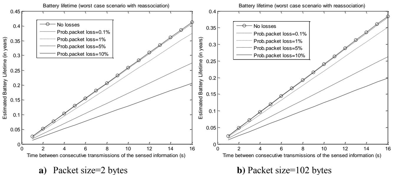
**Figure 11.** Effect of the re-association on the average battery consumption (Packet size = 2 bytes)
