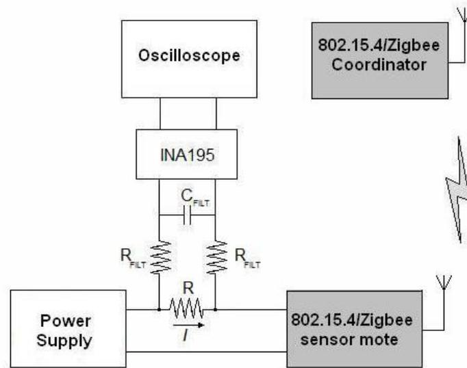
To design the value of  $R_{FILT}$ , we have to take into account that a high value can reduce the gain of the amplifier [32]:
