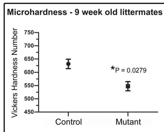
**Figure 5. *FoxO1* mutant enamel is softer than controls.** The Vickers microhardness test revealed that the adult *FoxO1* mutant teeth are significantly softer than their littermate controls.
