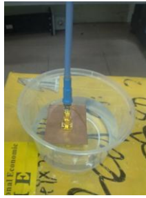
Fig. 3. Reflection measurement on water
