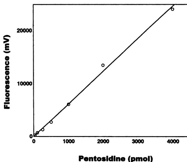
Fig. 3. Linear regression analysis of a calibration curve generated with seven calibrators prepared by adding pentosidine (40 pmol to 4 nmol) to 0.5 mL of urine.
