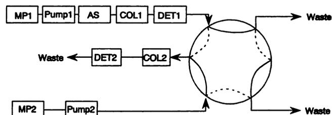
Fig. 1. HPLC system with a column-switching valve.
