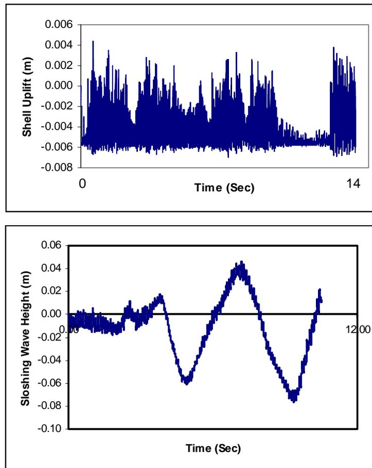
Figure 3. Typical time history response (a) Shell uplift (b) Liquid sloshing.
