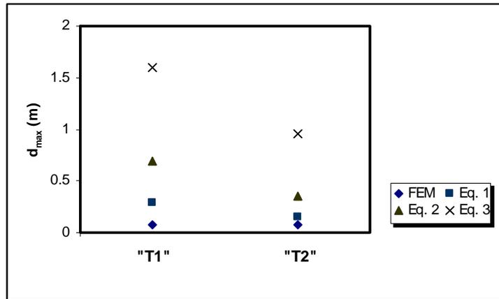
Figure 7. Predictions of Maximum sloshing wave heights by various methods.
