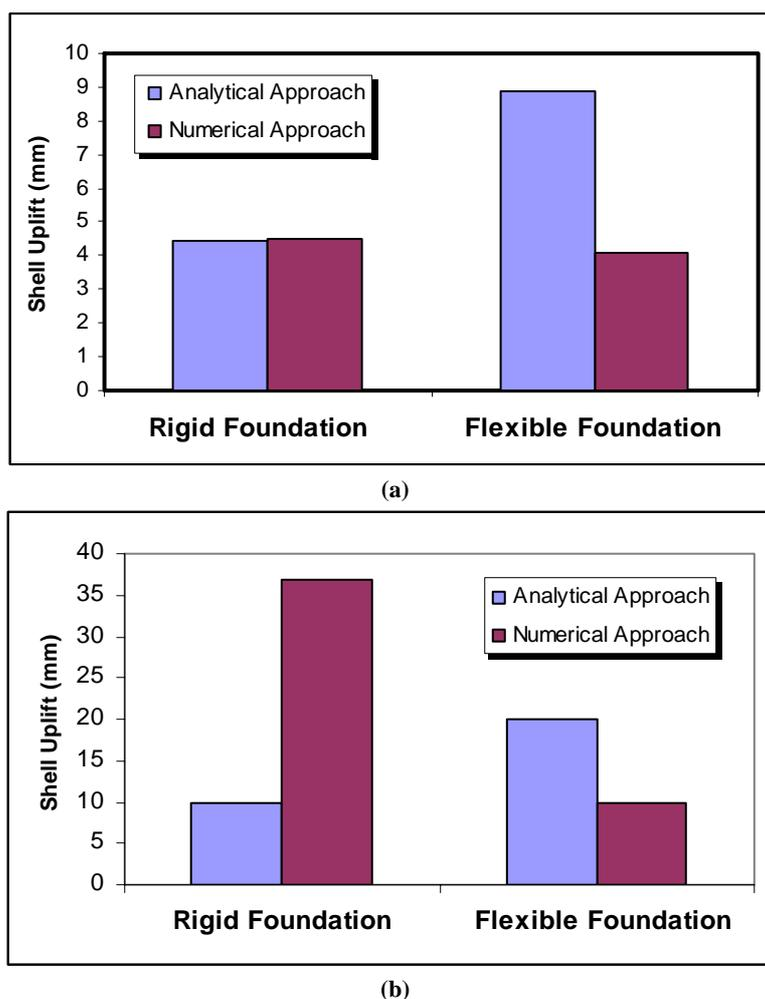
Figure 9. Comparison of shell uplift predict by finite element analysis and NZSEE method (a) Tank T1 (b) Tank T2.
