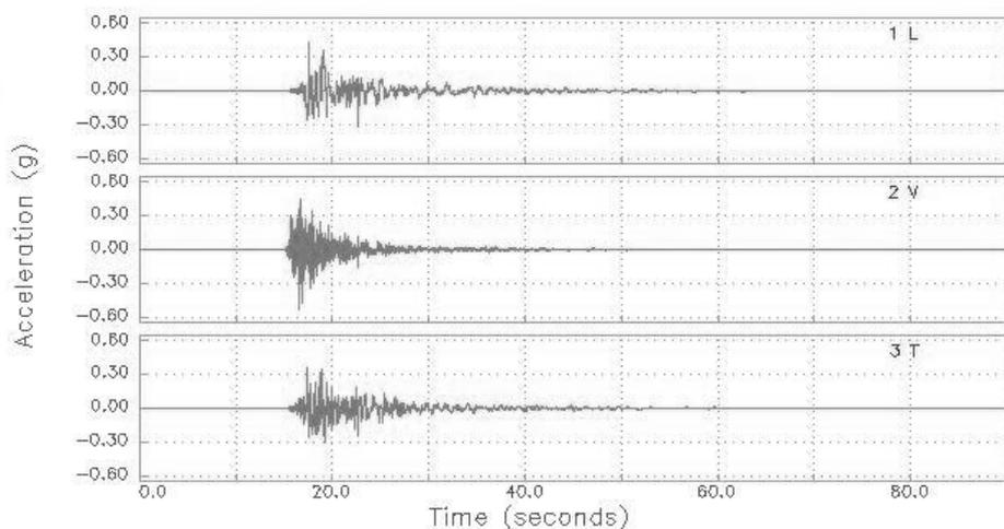
Figure 1. Accelerograms from Chalanchulan station (BHRC, 2006).
