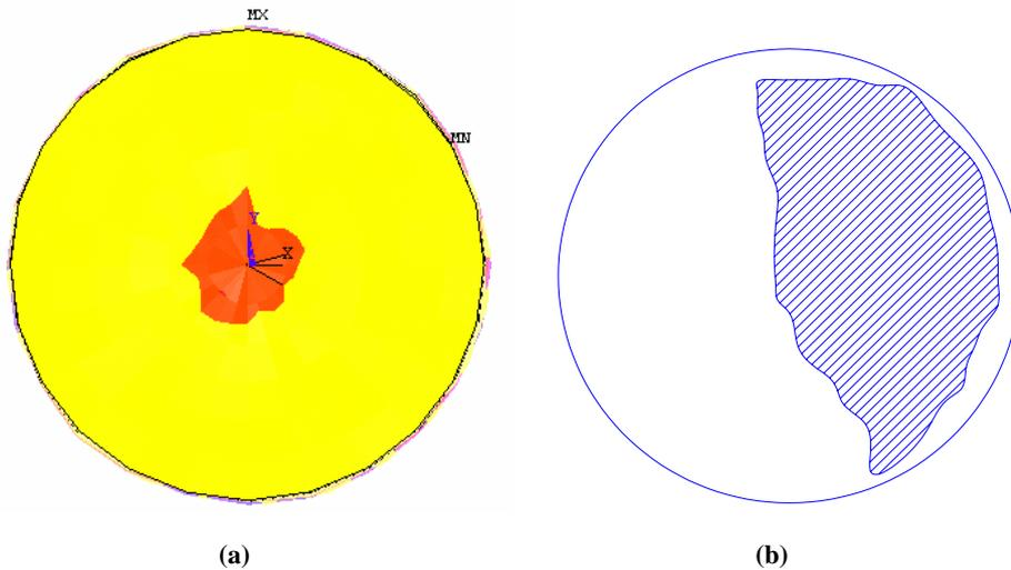
Figure 8. Comparison of roof distortions from finite element model with actual performance of tank T1 (a) FEM model (b) Schematic of observed damage.
