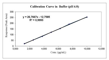
Fig. 5: Linearity on profils of dissolution test at pH 6.8
