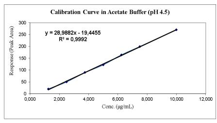
Fig. 4: Linearity on profils of dissolution test at pH 4.5
