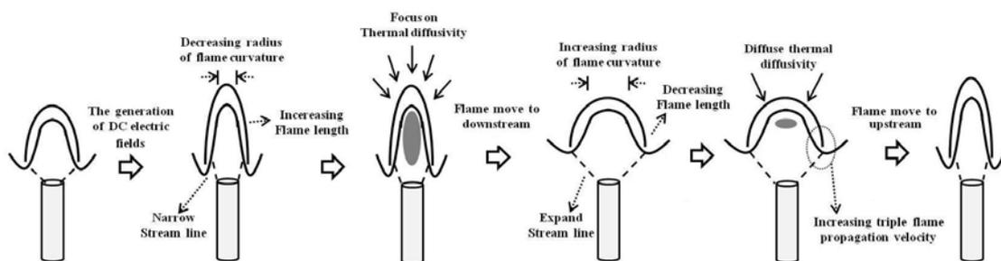
**Figure 4** Mechanism of diffusive-thermal instability in laminar jet flames.
