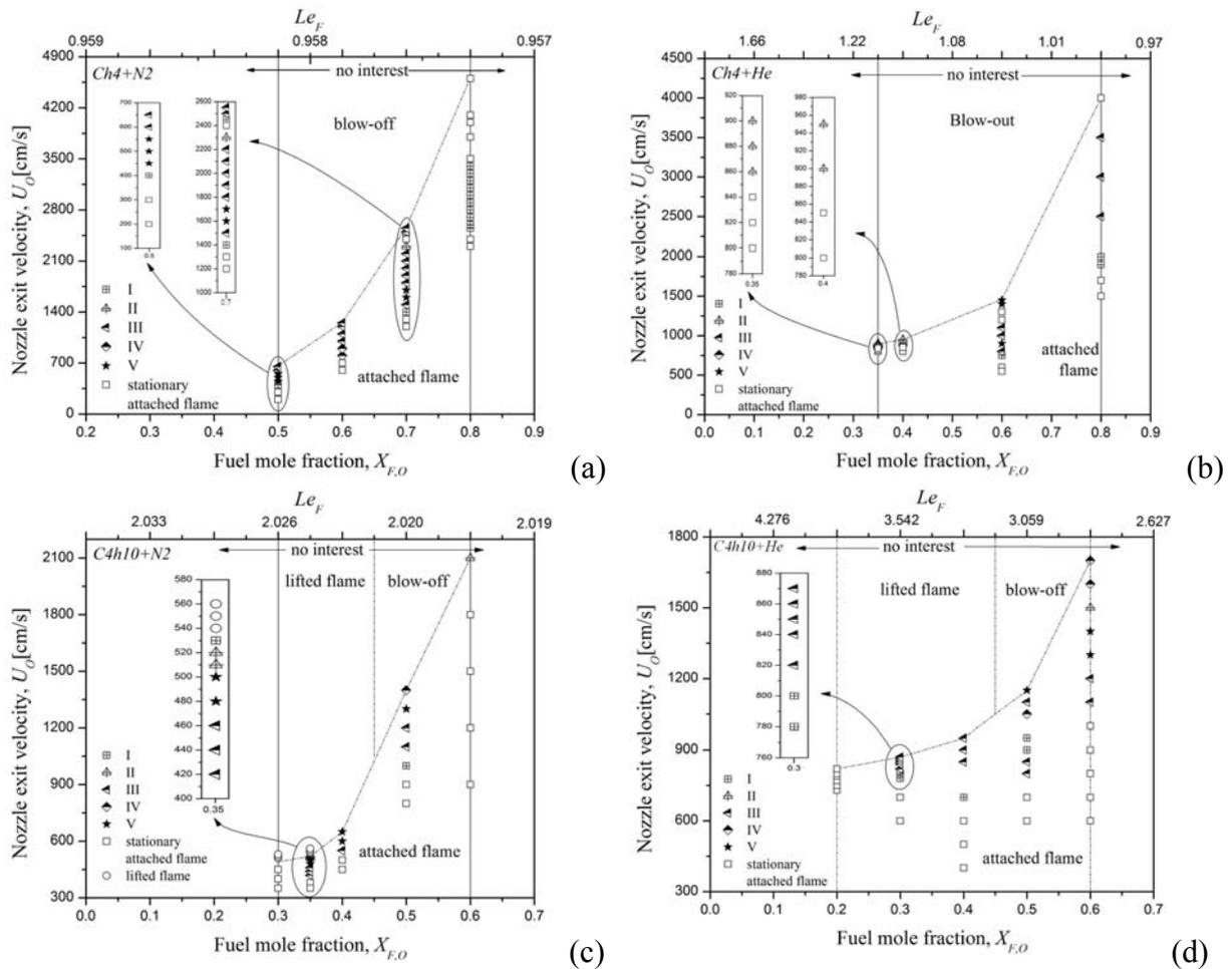
**Figure 5** Flame stability maps as a function of nozzle exit velocity and initial fuel mole fraction in vertically injected jet flames with (a)  $\text{CH}_4+\text{N}_2$ , (b)  $\text{CH}_4+\text{He}$ , (c)  $\text{C}_4\text{H}_{10}+\text{N}_2$  and (d)  $\text{C}_4\text{H}_{10}+\text{He}$ .
