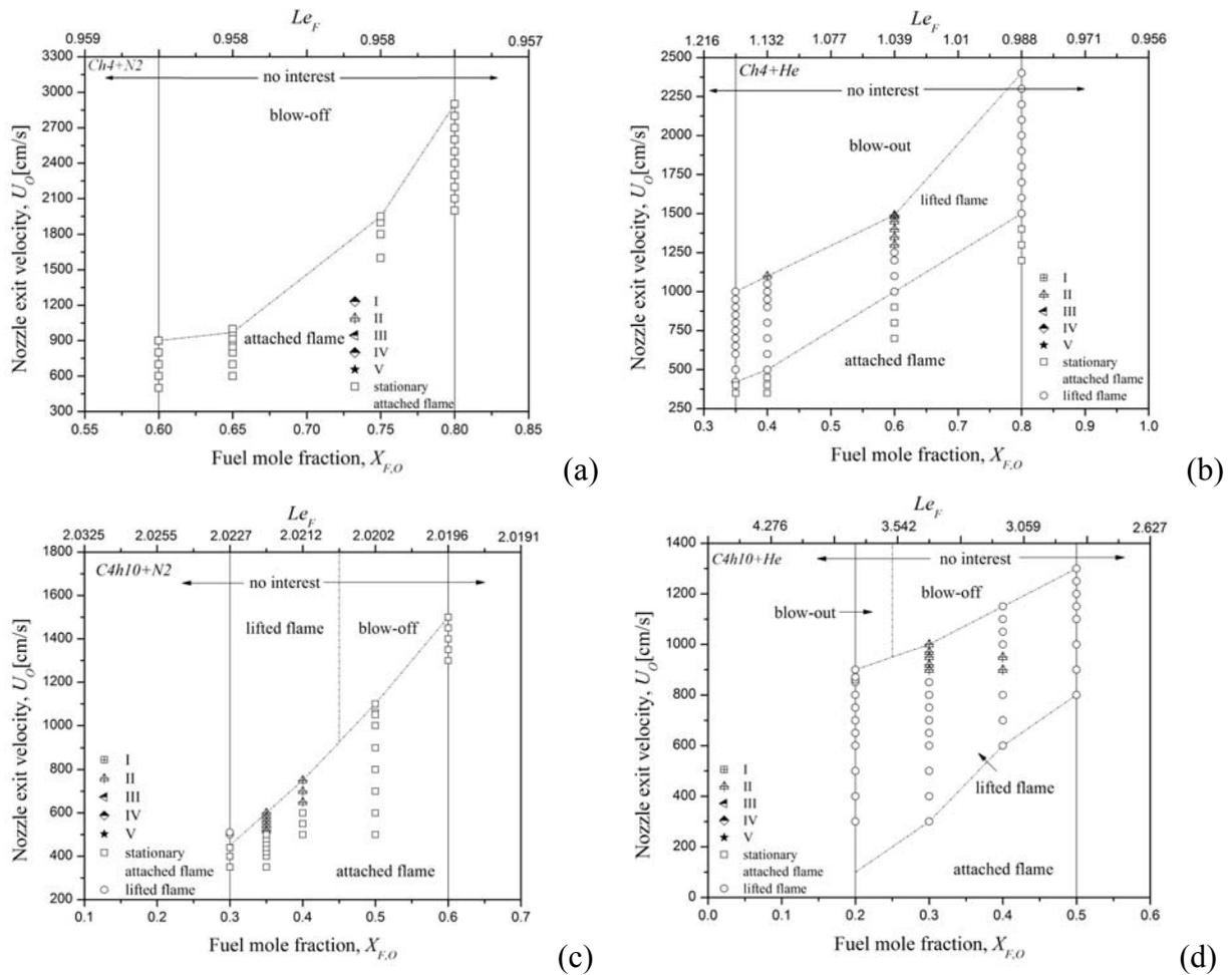
**Figure 2** Flame stability maps as a function of nozzle exit velocity and initial fuel mole fraction in horizontally injected jets with (a)  $\text{CH}_4+\text{N}_2$ , (b)  $\text{CH}_4+\text{He}$ , (c)  $\text{C}_4\text{H}_{10}+\text{N}_2$ , and (d)  $\text{C}_4\text{H}_{10}+\text{He}$ .
