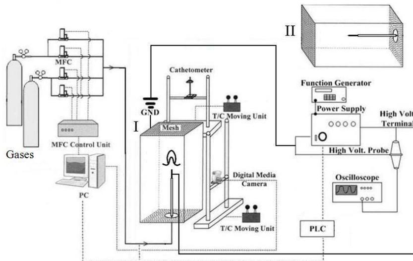
**Figure 1** Schematic of experimental setup: (I) vertical and (II) horizontal injections.
