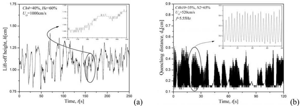
**Figure 3** Temporal variations of lift-off height at (a)  $X_{F,0} = 0.40$ ,  $U_0 = 1000\text{cm/s}$  for helium-diluted lifted methane jet flame and (b)  $X_{F,0} = 0.35$ ,  $U_0 = 520\text{cm/s}$  in nitrogen-diluted lifted butane jet flame.
