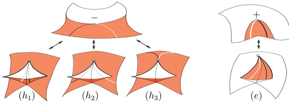
Figure 6: A godron of a smooth surface and its dual surface: a swallowtail.
