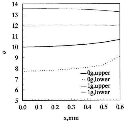
Fig. 6. Profiles of supersaturation at the upper and lower C/S interfaces in 1g and 0g cases after 1 h of crystal growth.
