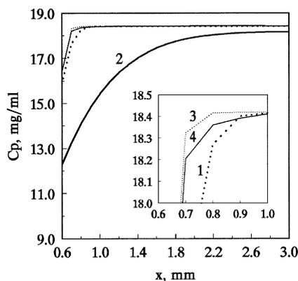
Fig. 5. Profiles of protein concentration in the solution at the half height of the crystal. The conditions corresponding to the curves are: curve 1— $0g$  and 1 min; curve 2— $0g$  and 1 h; curve 3— $1g$  and 1 min; curve 4— $1g$  and 1 h.
