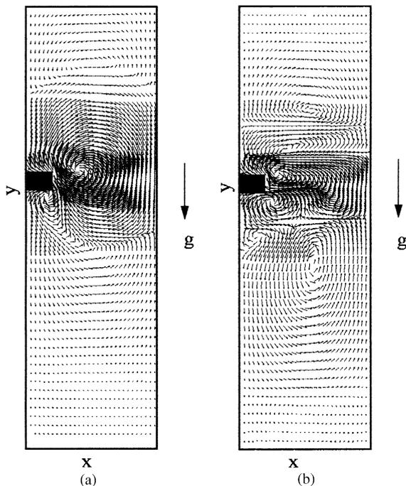
Fig. 3. Velocity vector fields of the solutal convection in  $1g$  case after (a) 1 s and (b) 1 h of crystal growth.
