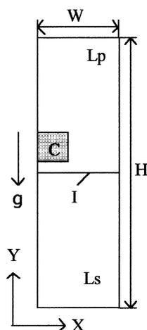
Fig. 1. Model of the liquid/liquid diffusion chamber,  $H = 20$  mm and  $W = 3$  mm. Symbols  $L_p$ ,  $L_s$ ,  $C$ ,  $I$  and  $g$  represent protein solution, salt solution, crystal seed, original interface and gravity acceleration, respectively.
