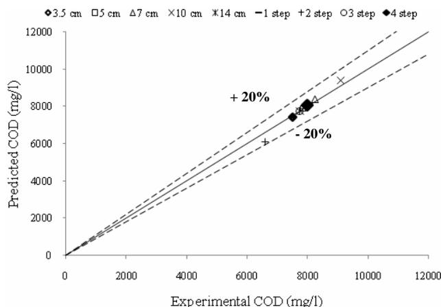
Fig. 7 Comparison of experimental and model-predicted COD
