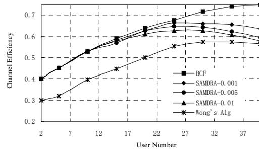
Figure 1. Channel Efficiency vs System Load
