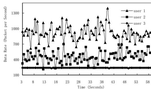
Figure 4. Data Rate for Different Channel Quality users As Function of Time
