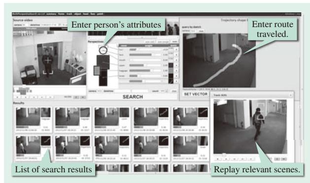
Fig. 5—User Screen for Multi-perspective Search. The screen displays the result of a search performed using attributes of the upper body, lower body, luggage, and route traveled as keys.
