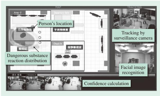
Fig. 3—Integrated Viewer. The viewer displays the location of people at a facility, estimated distribution of dangerous substances, surveillance camera video, and facial image recognition.
