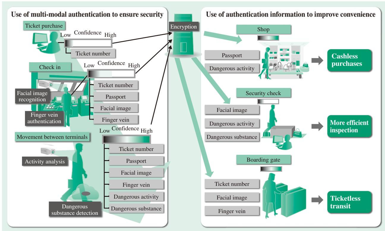
Fig. 1—Concept of Traceable Physical Security. The requirement is to combine use of multi-modal authentication for security with the use of the authentication information to improve convenience.
