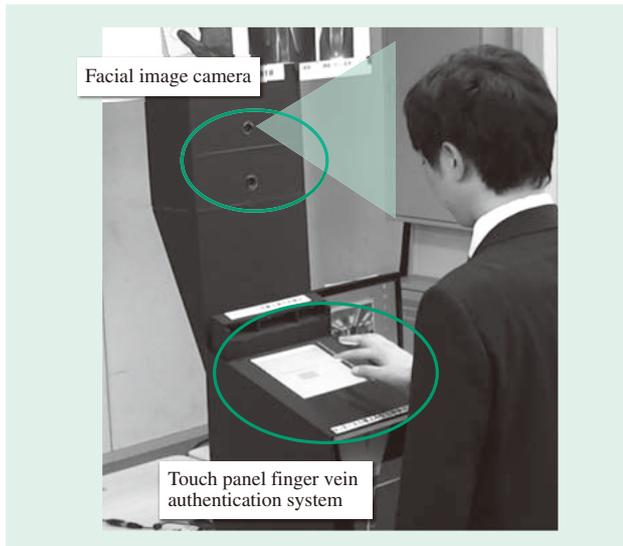
*Fig. 2—Touch Panel Finger Vein Authentication System. Finger vein authentication is performed while the user operates a touch panel, during which time a facial image is also captured.*
