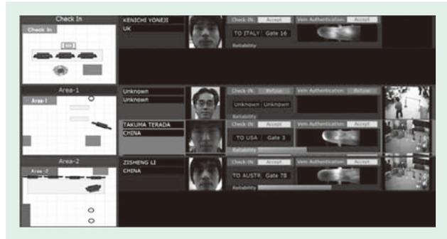
Fig. 4—Authentication Viewer. The screen displays authentication results from each area in turn.
