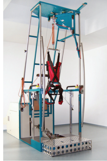
FIGURE 5: The Gangtrainer GT I (picture courtesy of Reha-Stim).
