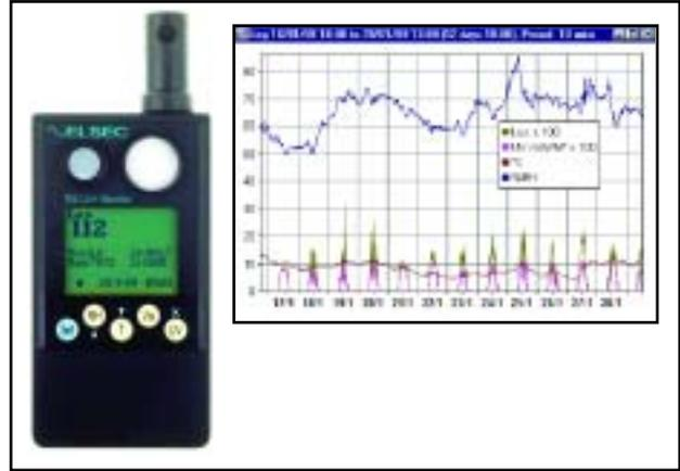
**Fig 6.** This UV-B meter, Elstec 743, continuously monitors radiation in the 290-400 nm wavelength spectrum. Such meters offer an economical method of assessing the value of UV-B lighting systems. The device also measures relative humidity, ambient temperature and visible light. Display from Elstec meter (inset).
