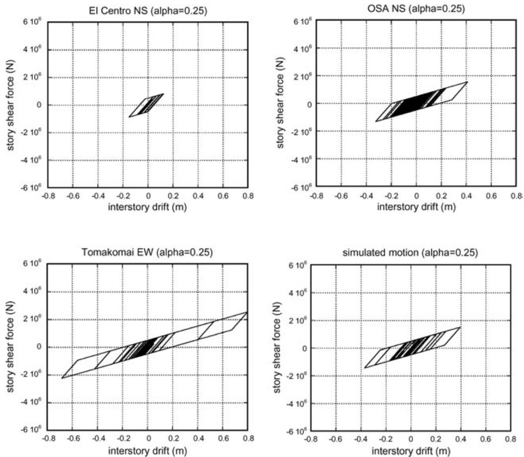
Figure 11. Restoring force characteristics in the BI system under four ground motions in the case of  $\alpha = 0.25$
