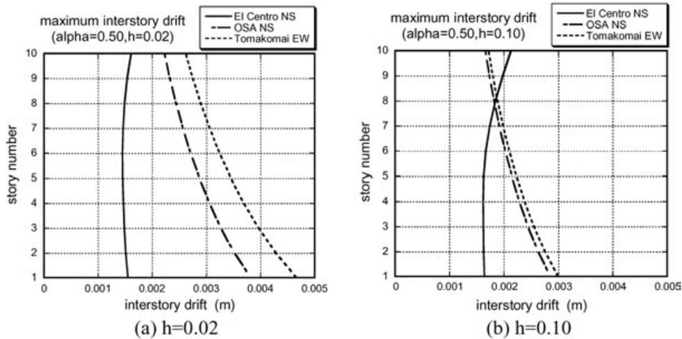
Figure 14. Maximum interstory drifts in the superstructure of the model with  $\alpha = 0.50$  under El Centro NS, OSA NS and Tomakomai EW for damping ratios 0.02 and 0.10 of the additional viscous damper
