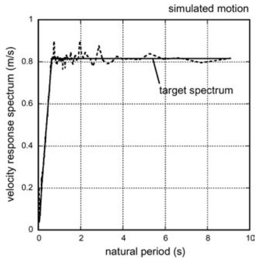
Figure 7. Compatibility of the velocity response spectrum of simulated motion with target spectrum (damping ratio 0.05)
