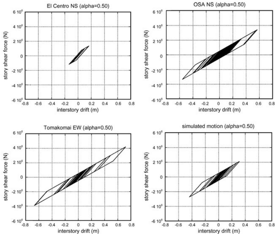
Figure 10. Restoring force characteristics in the BI system under four ground motions in the case of  $\alpha = 0.50$
