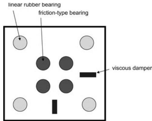
Figure 2. BI system consisting of linear rubber bearings, friction-type bearings and additional viscous dampers
