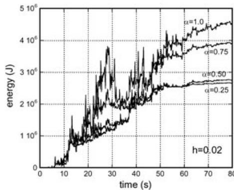
Figure 15. Time histories of input energies  $-\int_0^t \dot{\mathbf{u}}^T \mathbf{M} \mathbf{1} \ddot{u}_g d\tau$  to four models with different parameters  $\alpha = 0.25, 0.50, 0.75, 1.0$  by Tomakomai EW
