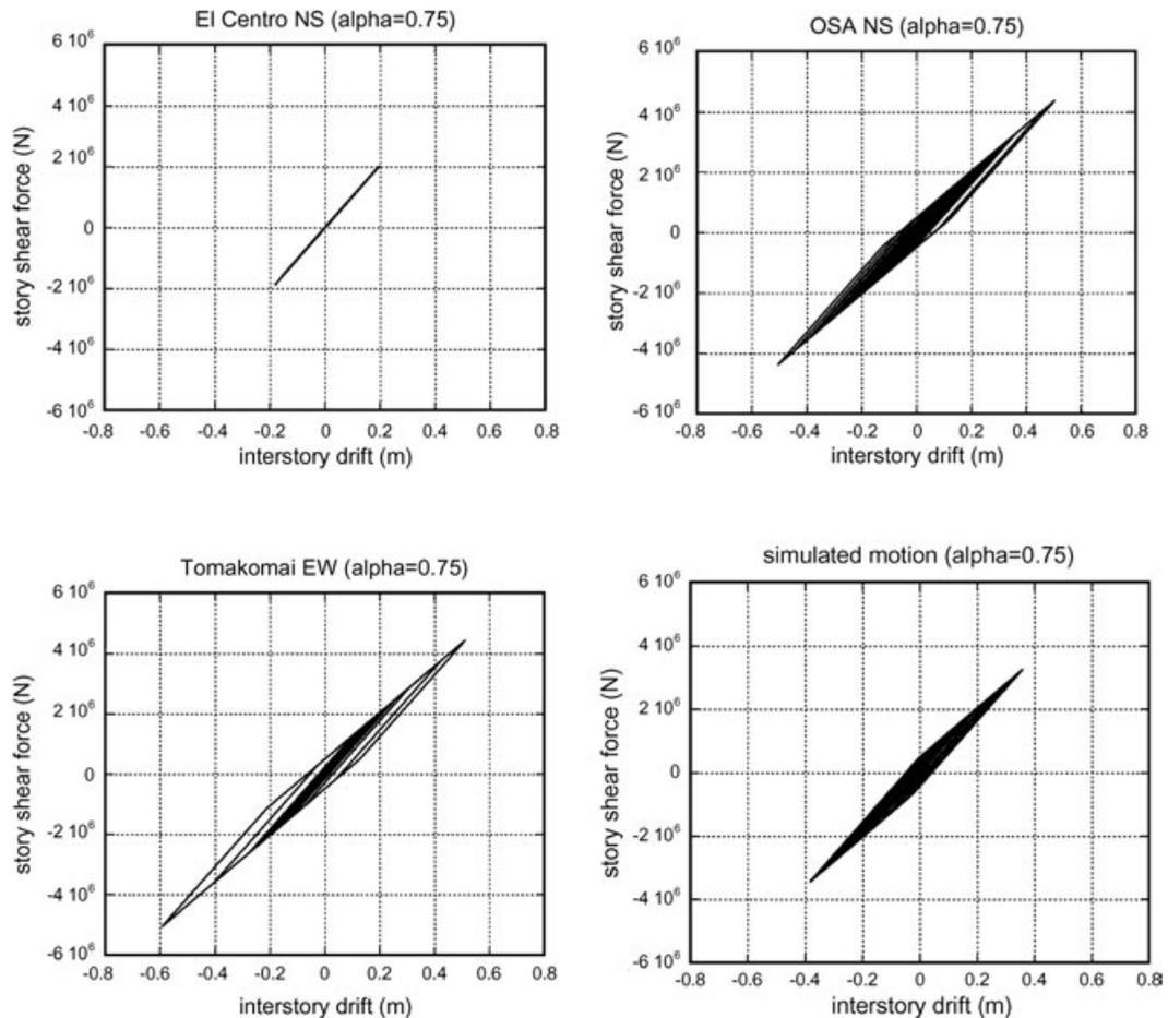
Figure 9. Restoring force characteristics in the BI system under four ground motions in the case of  $\alpha = 0.75$
