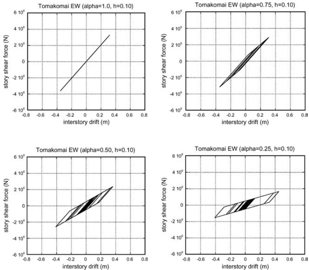
Figure 13. Restoring force characteristics in the BI system under Tomakomai EW for various  $\alpha$  values for the damping ratio 0.10 of the additional viscous damper
