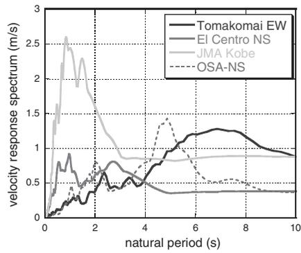
Figure 5. Velocity response spectra of four motions considered for damping ratio 0.05
