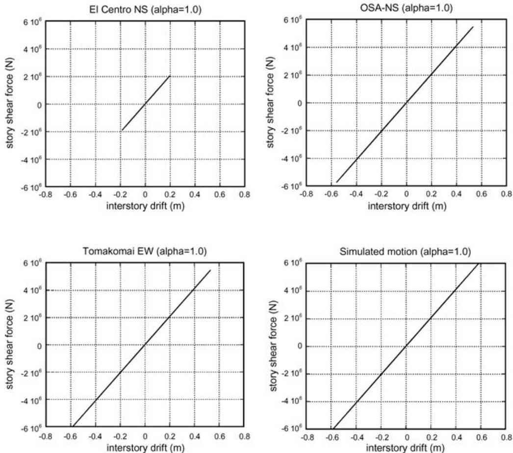
Figure 8. Restoring force characteristics in the BI system under four ground motions in the case of  $\alpha = 1.0$
