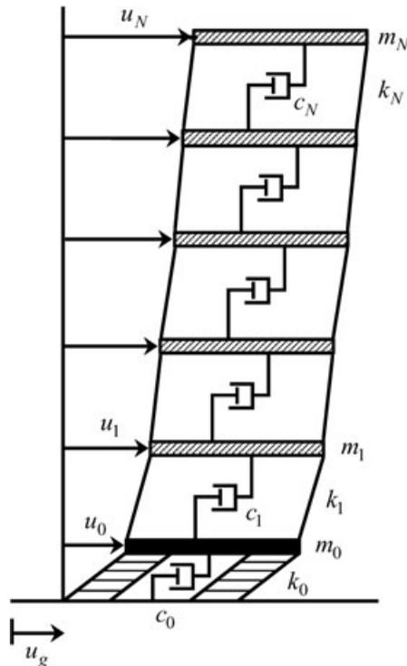
Figure 1.  $N$ -storey shear building model supported by a BI system
