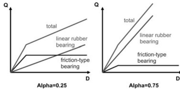
Figure 3. Restoring force characteristics of linear rubber bearing and friction-type bearing
