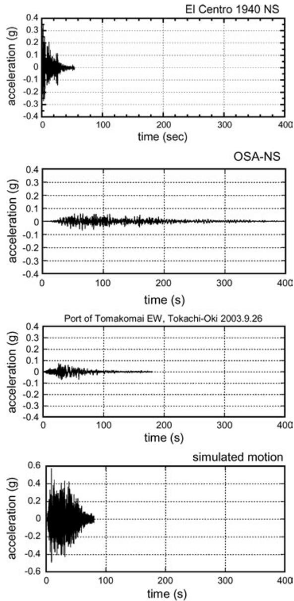
Figure 4. Acceleration records of El Centro NS (Imperial Valley, 1940), OSA NS (simulated Nankai Earthquake by Kamae *et al.*, 2004), Tomakomai EW (Tokachi-Oki, 2003) and a simulated motion compatible with the response spectrum of level 2 in the new Japanese Earthquake-resistant Design Code (2000)
