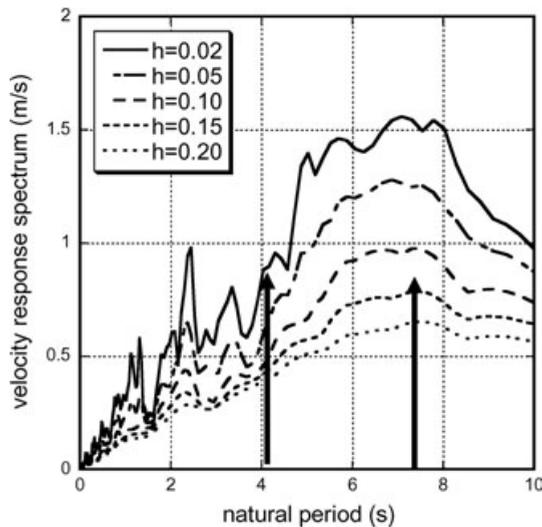
Figure 12. Velocity response spectra for various damping ratios for Tomakomai EW and the values for initial fundamental natural period (4.08 s) and equivalent fundamental natural period (7.25 s) for secant stiffness
