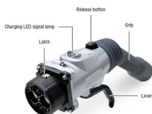
Figure 1: 10 pins CHAdeMO connector
