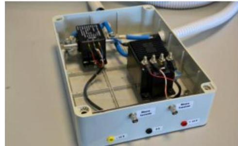
Figure 6: LEM DC output sensors
