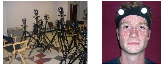
Figure 1: VICON system with eight cameras. The right panel shows an actor with the markers on the face and headband.
