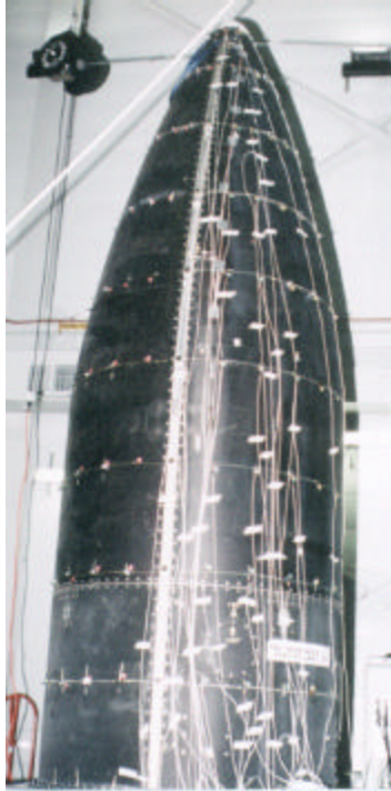
Figure 7. Structural modal testing of STARS fairing
