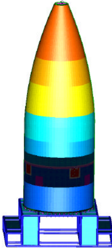
Figure 4. Structural Finite Element Model of STARS fairing and test stand
