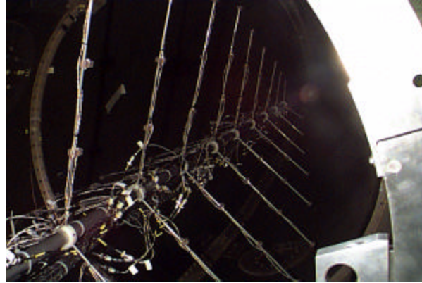
Figure 8. Microphone tree inside STARS fairing during acoustic modal testing
