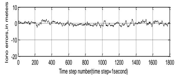
Fig. 5. The ionosphere delay error without Klobuchar model.
