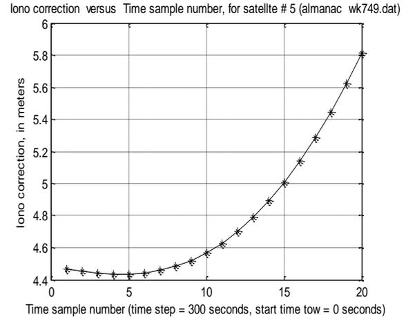
Fig. 3. Ionospheric correction of the 5<sup>th</sup> satellite
