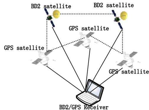
Fig. 1. Diagram of BD2/GPS combined system
