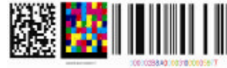
Figure 1. Samples of three different security printing deterrents: 2D barcode (left), color barcode with microtext (center) and 1D barcode (right).
