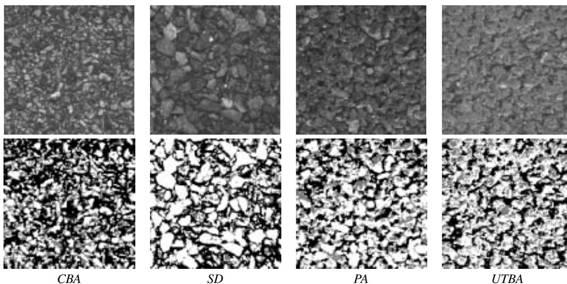
Figure 4: Example of simplified road texture images obtained for each surface category (white pixels  $\equiv$  Objects, black pixels  $\equiv$  Background and grey pixels  $\equiv$  Transitions).
