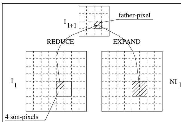
Figure 2: REDUCE and EXPAND operations. The lowest gray level *son*-pixel used to build *father*-pixel is represented by shaded area.
