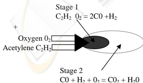
Figure 13: Oxy-Acetylene flame.
